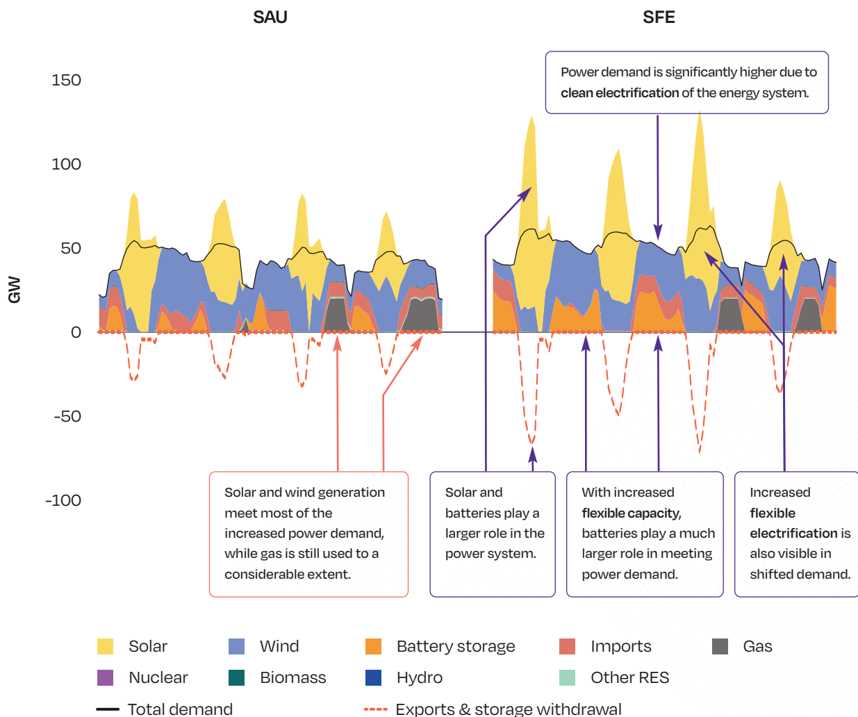
FIGURE 16 2040 POWER GENERATION AND CONSUMPTION PROFILES IN A REPRESENTATIVE SPRING WEEK IN THE NETHERLANDS, SAU SCENARIO VS SFE SCENARIO
